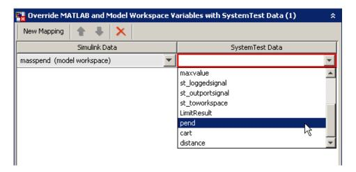
**4** Repeat steps 1 to 3 to override the Simulink model workspace variable penddistance with the SystemTest test vector distance.
