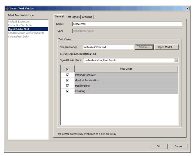
If there are any test cases you do not want to test, you can disable them using the check boxes. Test cases that are checked will be tested.
