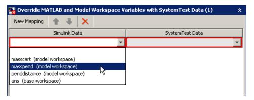
3 Specify which SystemTest test vector or test variable you want to map to the Simulink workspace variable. Click the SystemTest Data field of this row to see all available test vectors and test variables. For this example, select **pend**.
