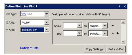
**Note** Selecting \*Auto\* when creating a plot means the plot will show the exact number of values in the test vector or result you are plotting. For example if you are plotting a test vector that has 50 values, and you select \*Auto\* for one of the axes, that axis will display 50 points.
