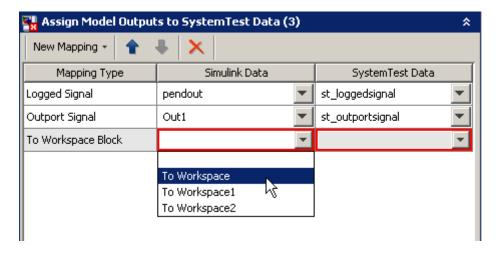
**3** Specify the SystemTest test variable to which you want to map the To Workspace block. Click the **SystemTest Data** field and select a test variable from the list. For this example, select **New Test Variable** to create a test variable.
