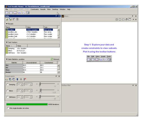
**Note** The most common use case is to have the Viewer open automatically after a test run, as described here. But you can also open the Viewer directly from MATLAB by typing stviewer at the MATLAB command line. The Viewer would open in an empty state. To open test results then, use the **File** > **Load Test Results** menu command.
