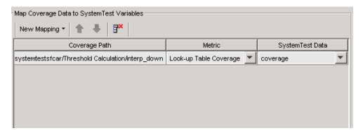
Note that if you select <New Test Variable> in the SystemTest Data column, the default name will match the input. For example, if the model name is system test pendulum from the Coverage Path column, and the metric you select in the **Metric** column is MCDC Coverage then the default name for the new variable would be system testpendulum mcdcinfo. The logical default name reflects the name of the model and the metric. You can use the default name or change it.
