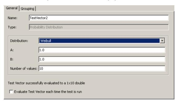
Weibull uses the function wblrnd and takes parameters for  $\boldsymbol{A}$  and  $\boldsymbol{B}$ .
