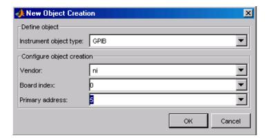
10 Click OK to return to the Edit: Instrument1 dialog box, where the instrument object is now filled in and selected for this resource (GPIBO-5).
