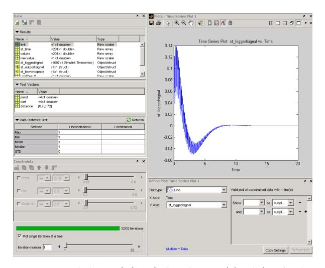
As this example shows, the time series test result for a single test iteration is composed of many values over time. There are many points with uneven spacing reflecting the actual values of the signal over the time period.
